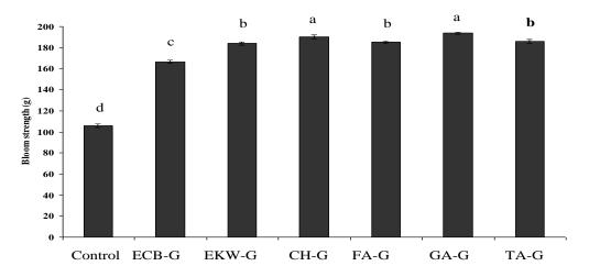
**Figure 2.** Gel strength of gelatin gel from cuttlefish skin incorporated with different oxidized extracts or commercial phenolic compounds. Bars represent the standard deviation (n=3). Different letters on the bars denote the significant differences (p<0.05). Control: without additives; ECB-G, EKW-G, CH-G, FA-G, TA-G, and GA-G: gelatin gel containing 2% oxidized ECB, EKW, catechin, ferulic acid, tannic acid, and gallic acid, respectively.
