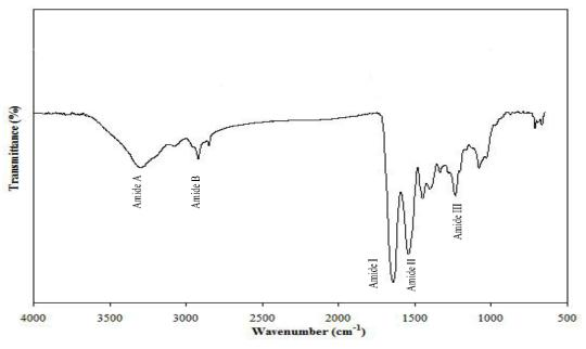
Figure 1. FTIR spectrum of gelatin powder extracted from cuttlefish skin.
